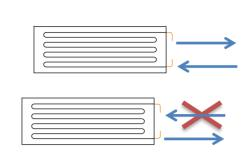
If the panel is installed at horizontal position, refrigerant inlet pipe should be connected into the bottom connection.
