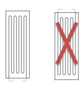
When the panel is installed in vertical position, always the inlet and outlet connection has been at the bottom. (It is not allowed to install the reverse)
